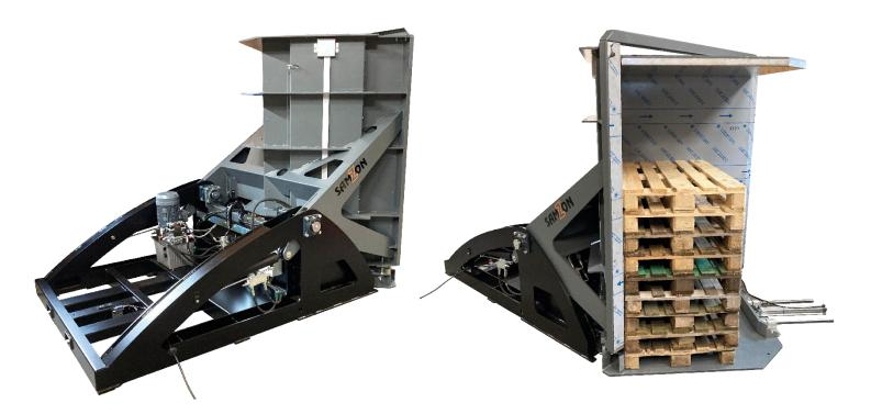
Capacity. Max 1400kg 2050/2450mm Hight Capacity Max. Hight Capacity Min. 680mm Required Room height. 3100mm / 3400mm Platform dim. 1200\*1200mm 1865mm (VT2000 / 1865mm (VT2400) Machine width. Machine length. 3670mm (VT2000 / 3942mm (VT2400) 2240mm (VT2000 / 2680mm (VT2400) Machine high. 1950kg / 2200kg Machine Weight. Operation. Manual / Automatic HMI Screen Cycle time. Approx. 25-30 pallets/hour 400V - 3 facers + N + PE - 50Hz Voltage.
