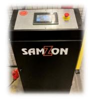
Samzon Pallet-Changer is a stationary machine for exchanging pallets without manual handling of the pallets. The pallet is fed into the machine using a pallet truck or pallet jack.
