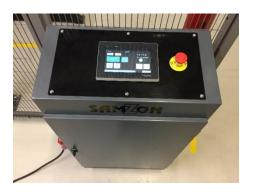
Samzon Pallet-Turner SD is a stationary pallet turner machine that is used to change pallets or for removing paper spacer or freezer spacer. The pallet is fed into the machine using a pallet truck or pallet jack. The machine can either rotate 90-degrees or 180-degrees depending on your needs. To remove paper spacer or freezer spacer, the machine is rotated from 0 to 90-degrees, pressure from the platforms is alleviated to allow for removal of spacers.
