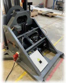
Samzon Pile-turner 104L is a stationary machine used for changing the pallet under a product. This model is often used in the paper-industry.
