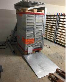
Samzon Pallet-inverter FL is a stationary pallet turner machine that runs to floor-level and is used to change pallets or for removing paper spacer or freezer spacer.
