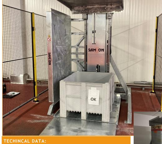
Capacity. MAX. 1500kg Hight Capacity MAX. 2000/2400mm Hight Capacity MIN. 500mm Platform dim. 1200\*1000mm Machine width. 1800mm (FL2000 / 2000mm (FL2400) 2200mm (FL2000 / 2400mm (FL2400) Machine length. 2800mm (FL2000 / 3200mm (FL2400) Machine high. Machine Weight. 1600kg / 1800kg Operation. Manual operated by bush button / auto by HMI screen Cycle time. Approx. 20-25 pallets/hour Voltage. 400V - 3 facers + N + PE
