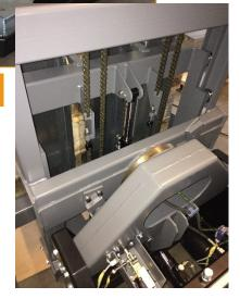
Samzon Pile-turner 104L pile-turner is a stationary machine used for changing the pallet under a product. This model is often used in the paper-industry.
