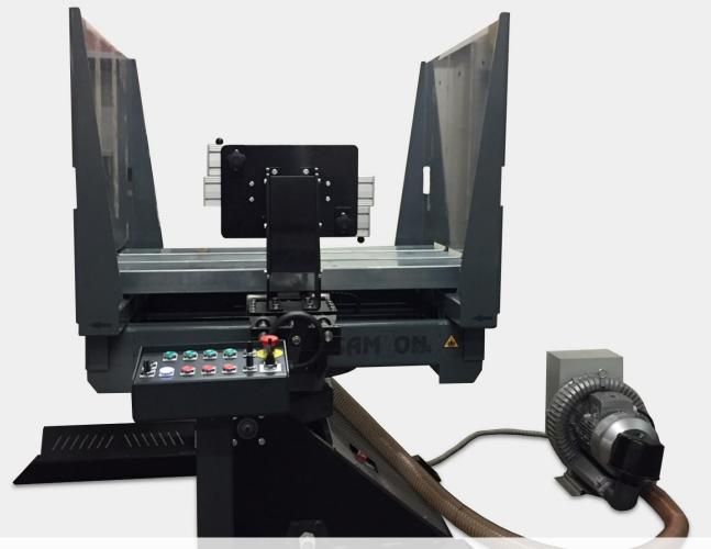
SAMZON pile turners are designed so that platforms can close down to 320mm; this allows short runs to be turned without the use of additional pallets. SAMZON is designed and manufactured in Denmark. The machine has low maintainence requirements and is equipped with top quality components.
