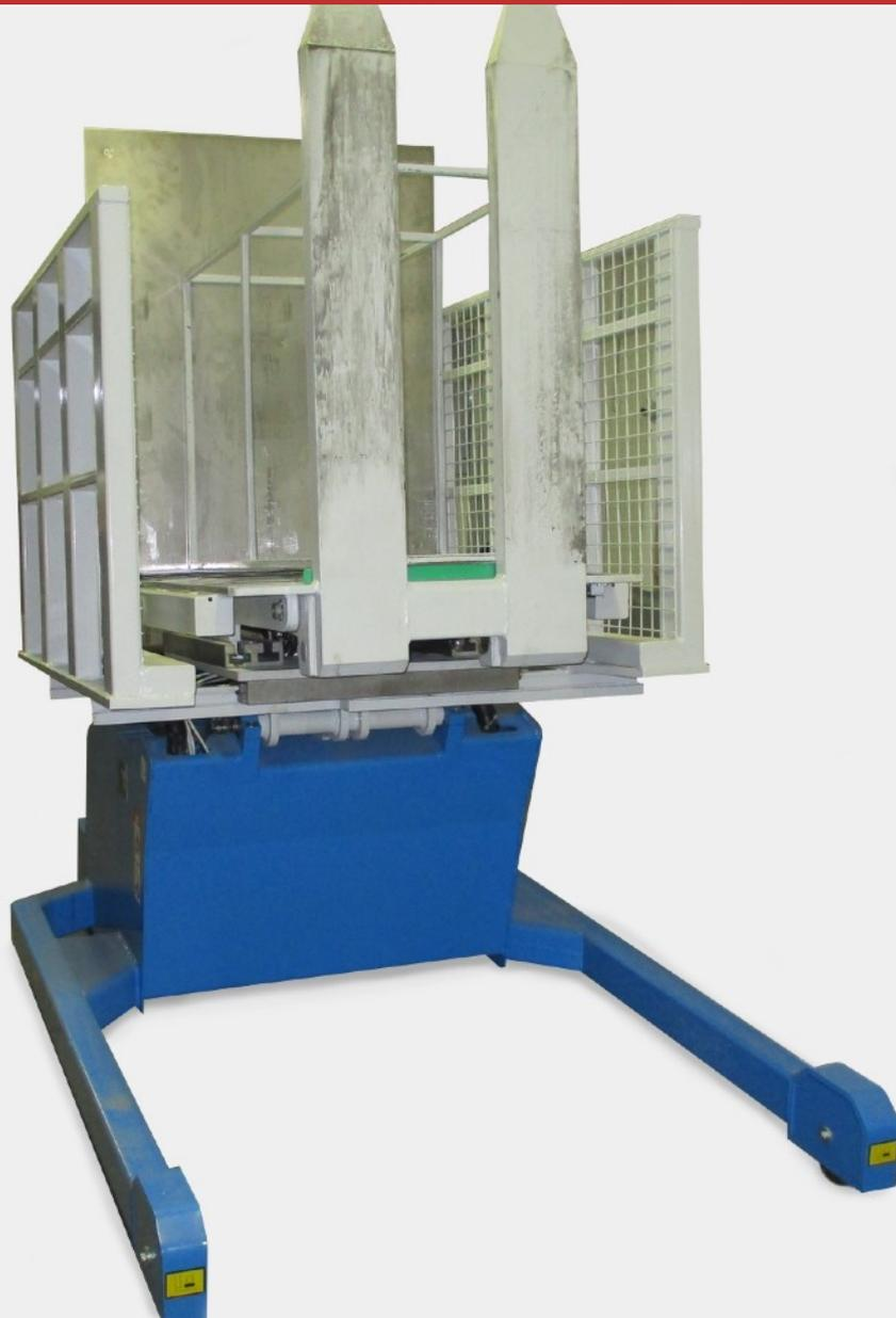
The pallet turner ARIES can count on the latest mechanical and electronic components. The traction group has a 1.300W electric engine, the oleo-dynamic has a 2.200W engine which includes a pump.
